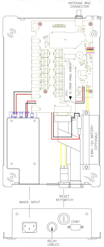
Note! When re-fitting the front panel ribbon cable, ensure that the connector collar is raised and check that the cable is square to the connector. Ensure that the cable runs straight in the direction shown. Gently insert the cable tail as far as it will go, then push down equally on both sides of the connector collar.
