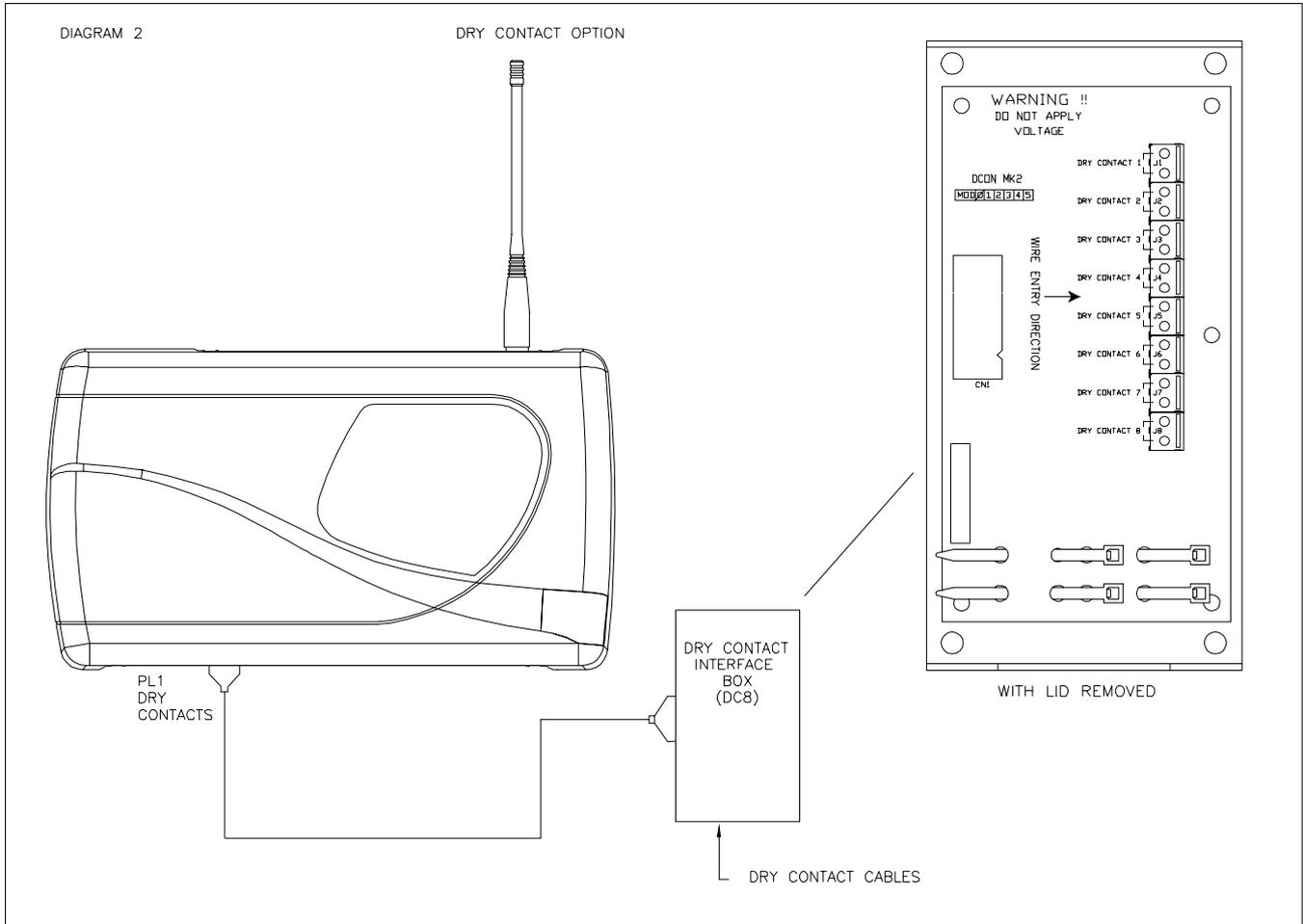
This option must be specified at time of ordering, along with the pre-programmed messages required. The purchaser should also order the dry contact interface box (Part Code: DC8) for ease of connection to the contact terminals (see Diagram 2).
